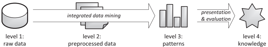
Figure 8: Enhanced KDD process by integrating the preprocessing step into the mining step for better handling of imperfect data
